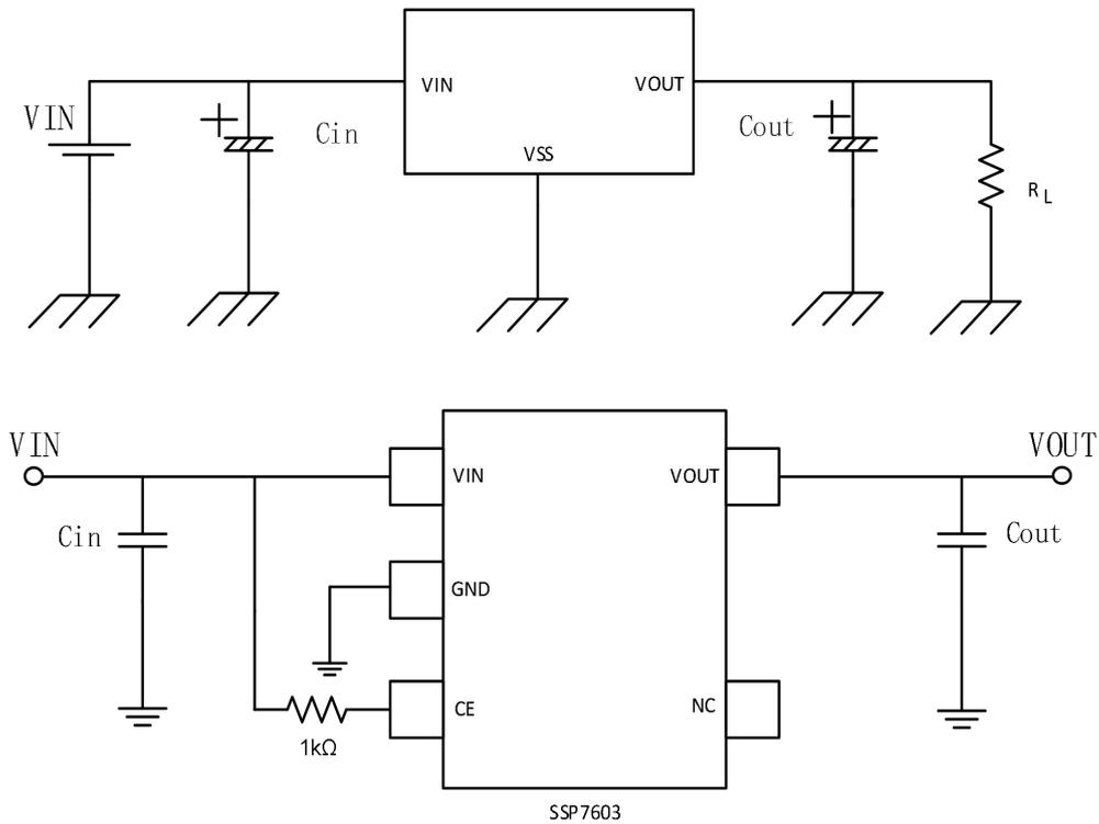
Note1: Input capacitor  $C_{in}=1\mu F$ .
